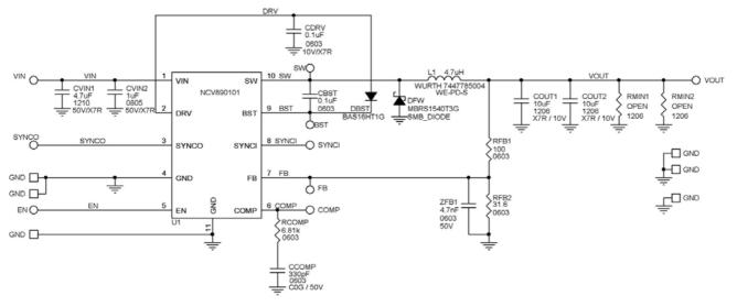
Figure 2. NCV890101GEVB Board Schematic
