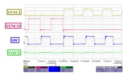
Figure 14. Starting synchronization at 2.5 MHz (from free-running)
