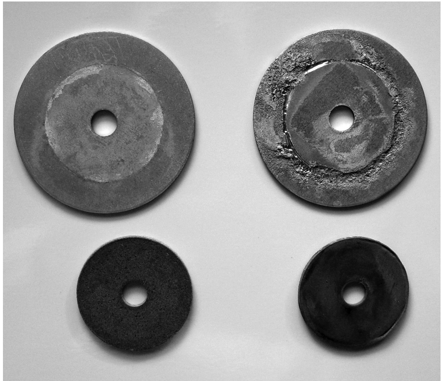
Comparison of corrosion results obtained from CHO-SEAL® 1298 conductive elastomer (left) and pure silver-filled elastomer (right) mated with aluminum after 168 hours of salt fog exposure.
