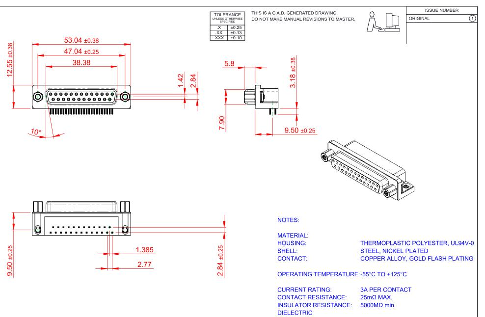
WITHSTANDING VOLTAGE: 1000V AC rms
