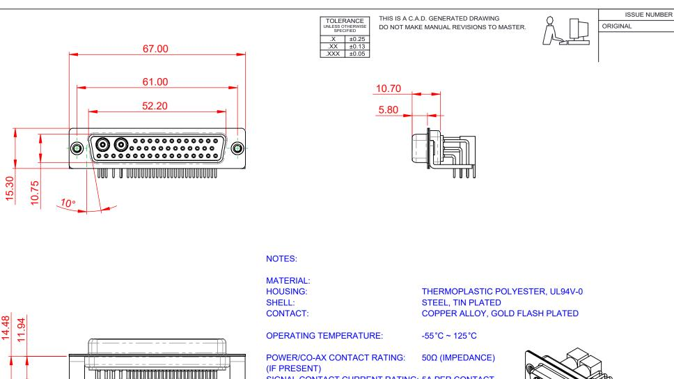
SIGNAL CONTACT CURRENT RATING: 5A PER CONTACT SIGNAL CONTACT RESISTANCE:  $10m\Omega$  MAX.
