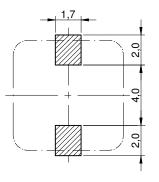
no sensitive traces underneath the component
