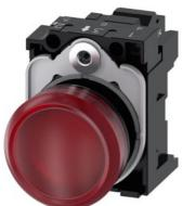
Indicator light, 22 mm, round, plastic, red, lens, smooth, with holder, LED module, with integrated LED 230 V AC, spring-type terminal, with laser labeling, upper case and lower case, always upper case at beginning of line
