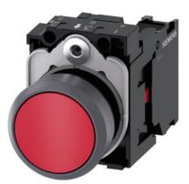
Pushbutton, 22 mm, round, plastic with metal front ring, red, pushbutton, flat, momentary contact type, with holder, 1 NC, screw terminal, with laser labeling, upper case and lower case, always upper case at the beginning of the word
