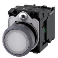
Illuminated pushbutton, 22 mm, round, plastic with metal front ring, white, pushbutton, flat, momentary contact type, with holder, 1NO, LED module with integrated LED 24 V AC/DC, screw terminal, with laser labeling, inscription or symbol Customer-specific selection with SIRIUS ACT configurator (CIN)
