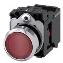
Illuminated pushbutton, 22 mm, round, metal, shiny, red, pushbutton, flat, momentary contact type, with holder, 1NC, LED module with integrated LED 24 V AC/DC, spring-type terminal, with laser labeling, lower case
