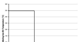
Soldering iron tip temperature should be set at 350°C (+10°C maximum), with the soldering duration not to exceed 3 seconds.
