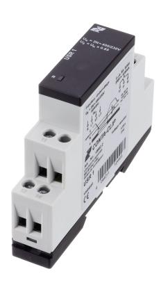
Undervoltage monitoring relay module with fixed switching threshold (195.5 V), Screw connection, Mounting type: Mounting rail TS 35, 1 CO contact
