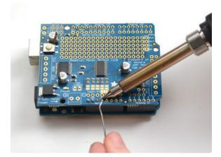
Solder each one of the pins into the shield to make a secure connection
