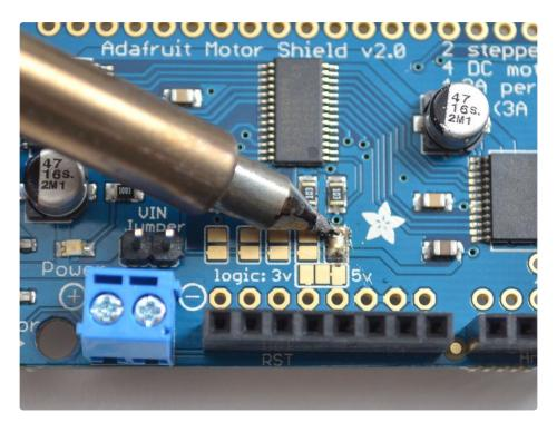
Board 0: Address = 0x60 Offset = binary 0000 (no jumpers required)
