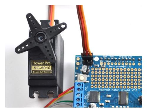
Hobby servos are the easiest way to get going with motor control. They have a 3-pin 0.1" female header connection with +5V, ground and signal inputs. The motor shield simply brings out the PWM output lines from Arduino pins 9 and 10 to two 3-pin headers so that its easy to plug in and go. They can take a lot of power so a 9V battery wont last more than a few minutes!
