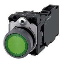
Illuminated pushbutton, 22 mm, round, plastic with metal front ring, green, pushbutton, flat, momentary contact type, with holder, 1 NO+1 NC, LED module with integrated LED 110 V AC, screw terminal
