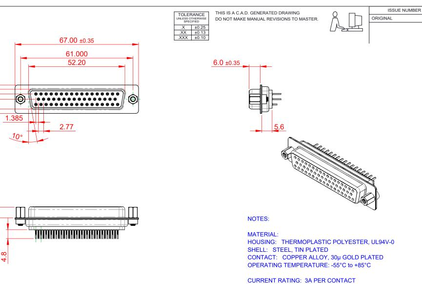
CONTACT RESISTANCE: 25mQ MAX. INSULATOR RESISTANCE: 5000MΩ min. DIELECTRIC WITHSTANDING VOLTAGE: 1000V AC rms (1)
