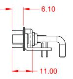
NOTES: MATERIAL: HOUSING: THERMOPLASTIC POLYESTER, UL94V-0 STEEL, NICKEL PLATED SHELL: CONTACT: COPPER ALLOY, GOLD FLASH PLATED 10.67 **OPERATING TEMPERATURE:** -55°C ~ 125°C 30A (CURRENT) POWER/CO-AX CONTACT RATING: (IF PRESENT) SIGNAL CONTACT CURRENT RATING: 5A PER CONTACT SIGNAL CONTACT RESISTANCE:  $10m\Omega$  MAX. Θ **INSULATOR RESISTANCE:** 5000MΩ min. DIELECTRIC Ø 0 0 WITHSTANDING VOLTAGE: 1000V AC rms 20.33
