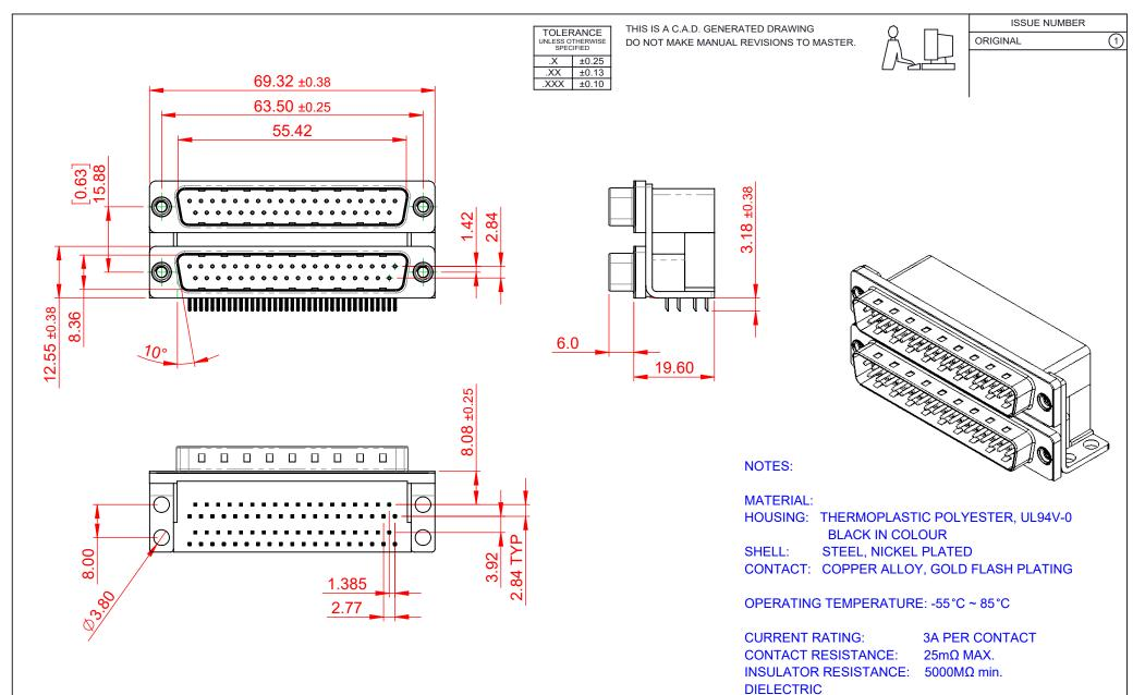
WITHSTANDING VOLTAGE: 1000V AC rms
