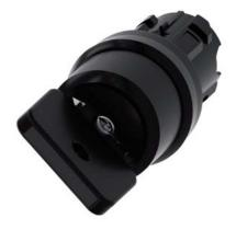
Key-operated switch O.M.R, 22 mm, round, plastic, lock number 73034, black, with 2 keys, 2 switch positions O-I, latching, actuating angle 90°, 10:30h/13:30h, key removal O+I, with laser labeling, upper case and lower case, always upper case at beginning of line
