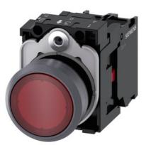
Illuminated pushbutton, 22 mm, round, plastic with metal front ring, red, pushbutton, flat, momentary contact type, with holder, 1NC, LED module with integrated LED 24 V AC/DC, screw terminal, with laser labeling, inscription or symbol Customer-specific selection with SIRIUS ACT configurator (CIN)
