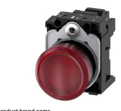
Indicator lights, 22 mm, round, plastic, red, lens, smooth, with holder, LED module, with integrated LED 230 V AC, spring-type terminal, with laser labeling, upper case and lower case, always upper case at the beginning of the word
