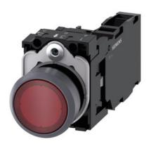
Illuminated pushbutton, 22 mm, round, plastic with metal front ring, red, pushbutton, flat, momentary contact type, with holder, 1 NO+1 NC, LED module with integrated LED 24 V AC/DC, screw terminal, with laser labeling, symbol number according to, ISO 7000 or IEC 60417
