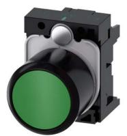
Pushbutton, compact, with extended stroke (12 mm), 22 mm, round, plastic, green, pushbutton, flat, momentary contact type, with holder, with laser labeling, upper case and lower case, always upper case at beginning of line
