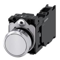
Pushbutton, 22 mm, round, metal, shiny, white, pushbutton, flat, momentary contact type, with holder, 1 NO+1 NC, spring-type terminal, with laser labeling, upper case and lower case, always upper case at beginning of line
