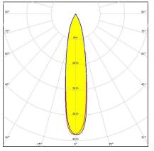
Dimensions: 111.0 mm x 111.0 mm Height: 80.00 mm ~18° smooth spot beam
