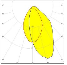
Dimensions: 111.0 mm x 111.0 mm Height: 37.00 mm Asymmetric beam for wall-washing
