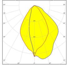
Dimensions: 111.0 mm x 111.0 mm Height: 32.60 mm White version with asymmetric beam for wall-washing
