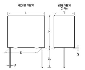
**General Information** Series F612 Dielectric Metallized Polyester Stacked Style Radial MKT (Stacked), DC Multipurpose Applications Features RoHS Yes Lead Wire Leads AEC-Q200 No Component 0.23 g Weight The Rated Voltage Decreases 1.25%/C Between +85C And +105C (For +125C, Please Consult KEMET). ClimCat: 55/105/56. Miscellaneous
