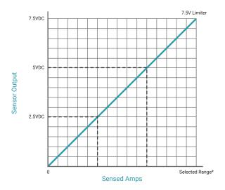
\*Factory calibrated ranges selected with the amperage range switch
