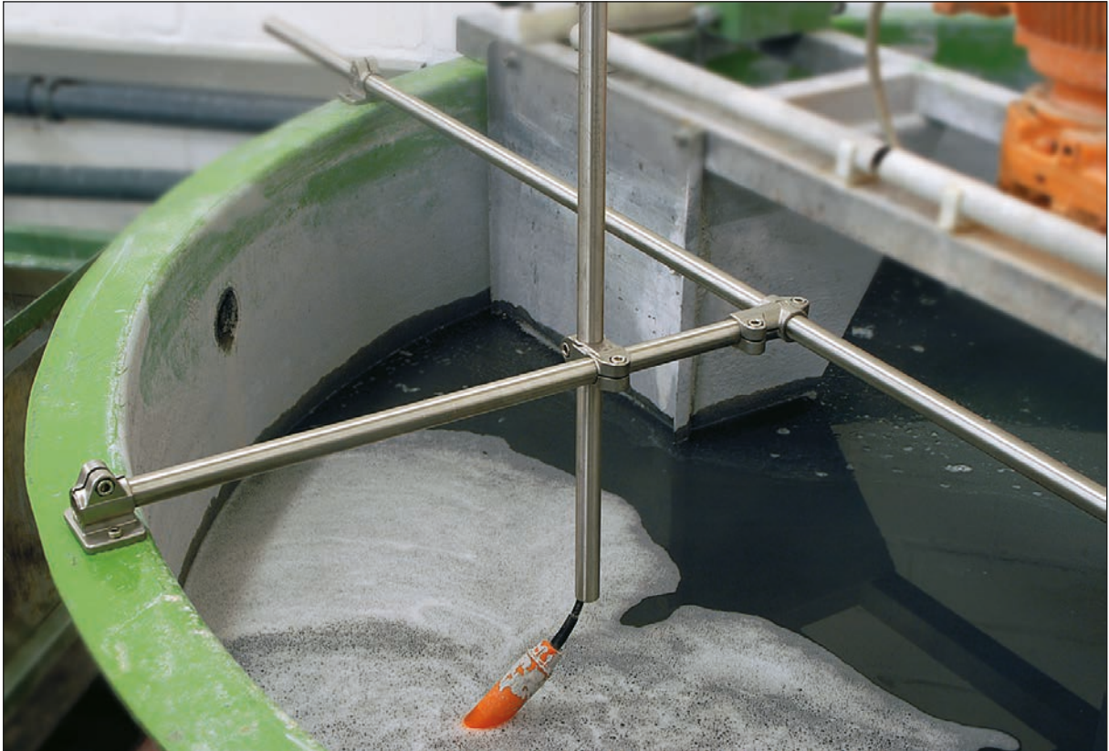
Simple probe fixation in an aggressive environment.
