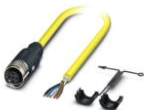
Sensor/actuator cable, 5-position, PVC, yellow, shielded, free cable end, on Socket straight M12 SPEEDCON, A-coded, cable length: 5 m
