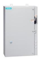
Non-reversing motor starter, Size 1 3/4, Three phase full voltage, Solidstate overload relay, OLR amp range 10-40A, 24VAC 50-60Hz coil, Combination type, 60A non-fusible disconnect, Encl NEMA type 4X 304 S-Steel, Water/dust tight noncorrosive, Extra-wide enclosure
