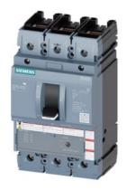
circuit breaker 3VA5 UL frame 250 3-pole, starter protection TM120M, AM, In=150A without overload protection short-circuit protection Ii=3...6 x In cable connection on both sides
