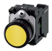
Pushbutton, 22 mm, round, plastic, yellow, pushbutton, flat, momentary contact type, with holder 1 NO, spring-type terminal, with laser labeling, upper case and lower case, always upper case at beginning of line
