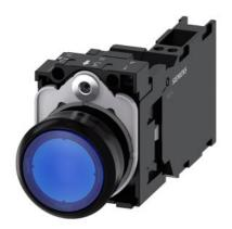
Illuminated pushbutton, 22 mm, round, plastic, blue, pushbutton, flat, momentary contact type, with holder, 1 NO+1 NC, LED module with integrated LED 24 V AC/DC, spring-type terminal, with laser labeling, lower case
