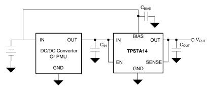
Figure 8-4. High-Efficiency Supply From a Rechargeable Battery
