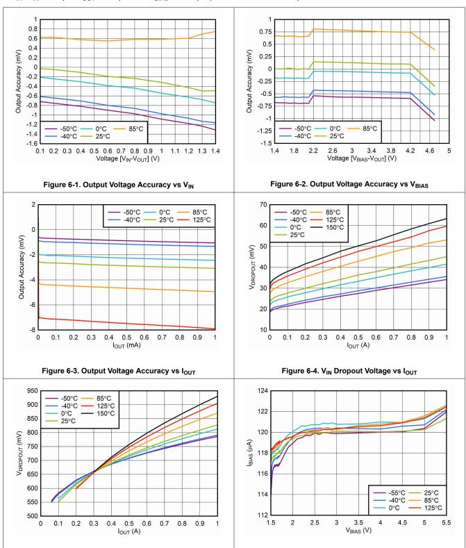
Figure 6-5. V<sub>BIAS</sub> Dropout Voltage vs I<sub>OUT</sub>
