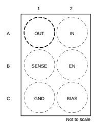
Figure 5-1. YBK Package, 6-Pin WCSP (Top View)
