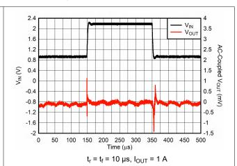
Figure 6-20. Line Transient From 1 V to 2.2 V
