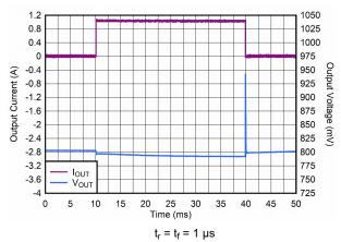
Figure 6-21. Load Transient From 100 µA to 1 A
