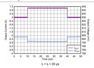
Figure 6-22. Load Transient From 100  $\mu A$  to 1 A
