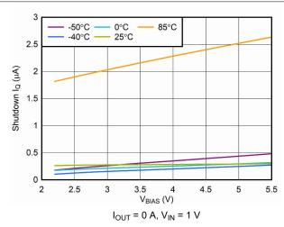
Figure 6-9. V<sub>BIAS</sub> Shutdown I<sub>Q</sub> vs V<sub>BIAS</sub>
