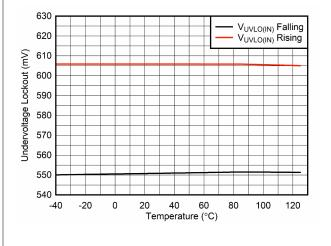
Figure 6-12.  $V_{\rm IN}$  UVLO vs Temperature
