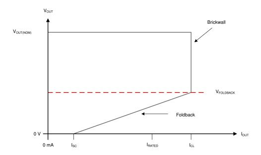
Figure 7-2. Foldback Current Limit
