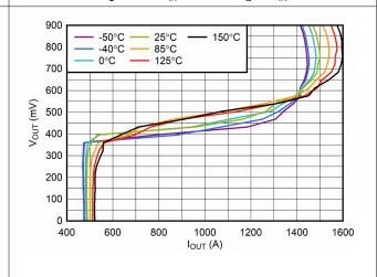
Figure 6-10. V<sub>OUT</sub> Foldback Current Limit vs Output Current
