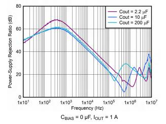
Figure 6-24. PSRR vs Frequency and Cout
