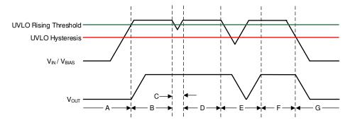
Figure 8-2. Typical V<sub>IN</sub> or V<sub>BIAS</sub> UVLO Circuit Operation
