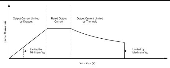
Figure 8-3. Continuous Operation Diagram With Description of Regions
