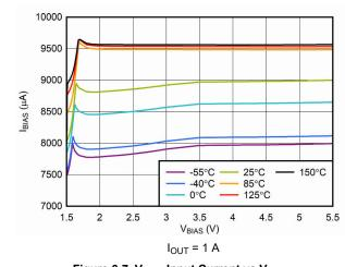
Figure 6-7.  $V_{\text{BIAS}}$  Input Current vs  $V_{\text{BIAS}}$
