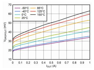
$V_{BIAS} = V_{OUT(NOM)} + 1.4 \text{ V}, V_{EN} = V_{IN}, C_{IN} = 2.2 \ \mu\text{F}, C_{OUT} = 2.2 \ \mu\text{F}, and } C_{BIAS} = 0.47 \ \mu\text{F}$
