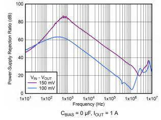
Figure 6-23. PSRR vs Frequency and  $V_{\text{IN}}$  –  $V_{\text{OUT}}$
