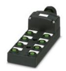
Sensor/actuator box, application: Standard, connection method: M12-SPEEDCON-socket Plastic, number of slots: 8, number of positions: 5, coding: A - standard, slot assignment: Double, status display: No, Universal; master cable connection: Pluggable screw connection 180°, shielding: no
