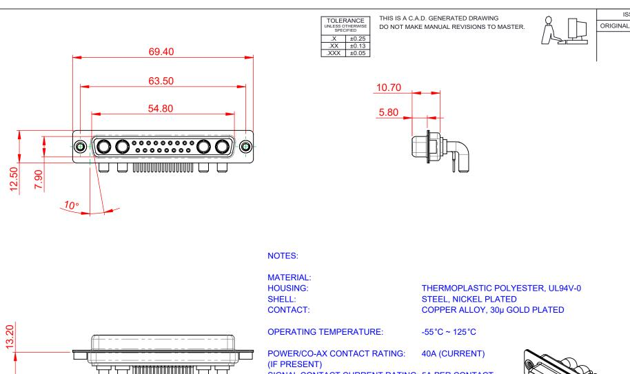
SIGNAL CONTACT CURRENT RATING: 5A PER CONTACT SIGNAL CONTACT RESISTANCE:  $10m\Omega$  MAX.
