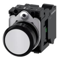
Pushbutton, 22 mm, round, plastic, white, pushbutton, flat, momentary contact type, with holder 1 NO, spring-type terminal, with laser labeling, symbol number according to, ISO 7000 or IEC 60417
