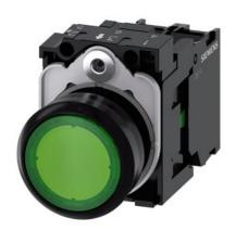
Illuminated pushbutton, 22 mm, round, plastic, green, pushbutton, flat, momentary contact type, with holder, 1NO, LED module with integrated LED 24 V AC/DC, screw terminal, with laser labeling, lower case
