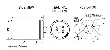
General Information Series ALC70 Dielectric Aluminum Electrolytic Description Snap-In, Aluminum Electrolytic RoHS Lead 3 Pin Short AEC-Q200 No Halogen Free Yes Component Weight 165 g Notes Dimensions D And L Include Sleeving. Shelf Life 156 Weeks
