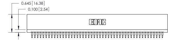
745 Series Ultra-Mate Card Edge Connector - Press Fit Part Number: 745-047-525-101
