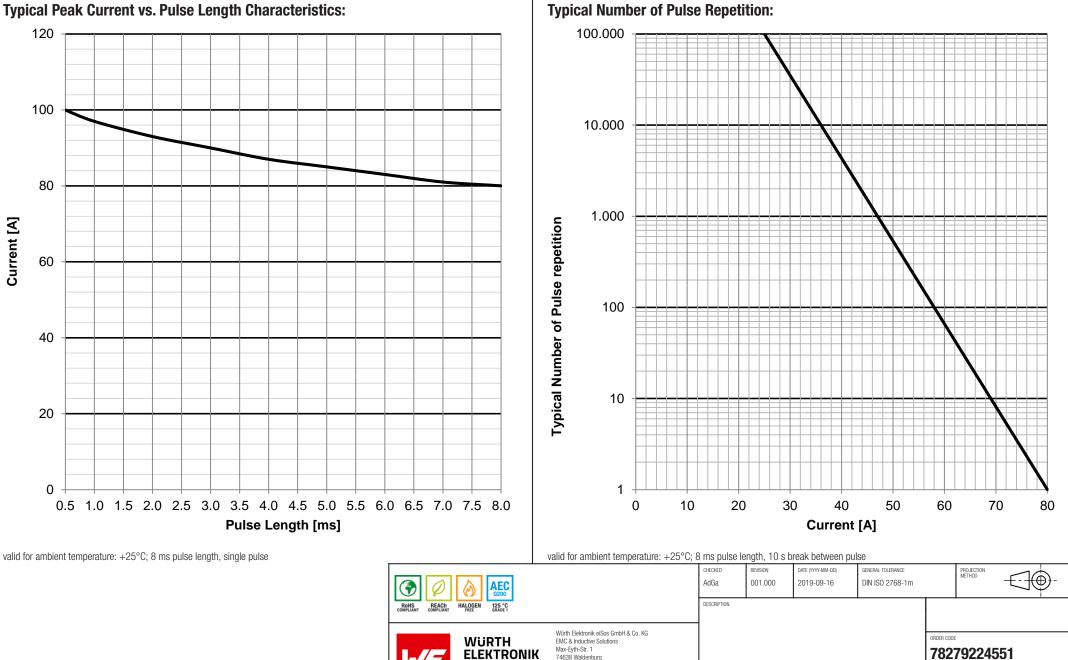
**Typical Peak Current vs. Pulse Length Characteristics:**
