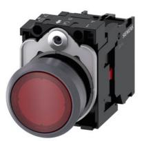
Illuminated pushbutton, 22 mm, round, plastic with metal front ring, red, pushbutton, flat, momentary contact type, with holder, 1NC, LED module with integrated LED 110 V AC, screw terminal, with laser labeling, symbol number according to, ISO 7000 or IEC 60417
