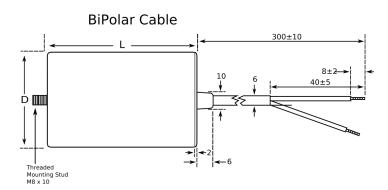
General Information Series C27 Dielectric Film/Foil Polypropylene Style Plastic Case and Cover, Ultra Sonically Welded Description Ultra Sonically Welded Seal, Safety Class PO, UL\_94 VO Disk **Features** RoHS Yes Termination Tin Copper Lead BiPolar Cables UL, VDE, UL (Construction Only), UL\_94 VO Disk Qualifications AEC-Q200 Component 39.08 g Weight
