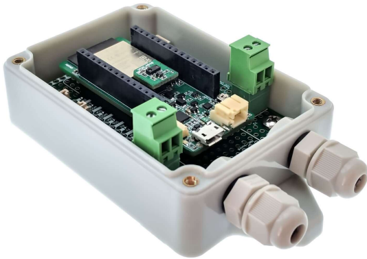
Pic. 22. WiFi ToF sensor : waste collection project
