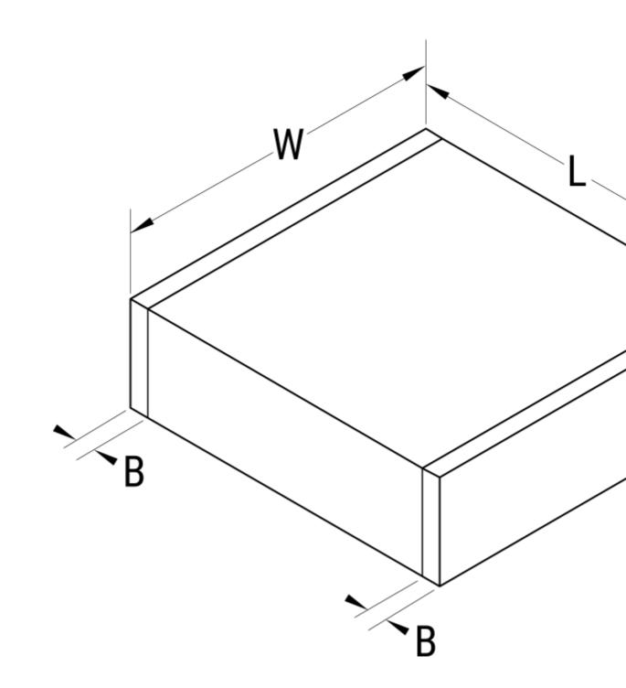
Click here for the 3D model. Dimensions Chip Size 1210 L 3.3mm +0.3/-0.1mm
