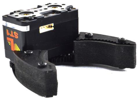
The gripper is made of durable aluminum plates and standoffs and uses foam to conform to the object being grasped. Inner teeth on the aluminum help "bite" into objects when necessary. Alternatively, 3D print your own inserts to customize the gripper for your robotic application.
