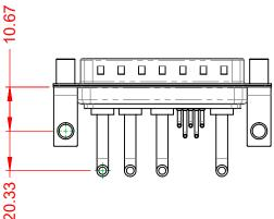
20A (CURRENT) POWER/CO-AX CONTACT RATING: (IF PRESENT) SIGNAL CONTACT CURRENT RATING: 5A PER CONTACT SIGNAL CONTACT RESISTANCE:  $10m\Omega$  MAX. **INSULATOR RESISTANCE:**
