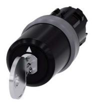
key-operated switch Siemens, 22 mm, round, plastic with metal front ring, lock number SSG10, with 2 keys, 3 switch positions I>O<II, momentary contact type, actuating angle 2x45°, 10:30h/12h/13:30h, key removal O, with laser labeling, inscription or symbol customer-specific selection with SIRIUS ACT configurator (CIN)
