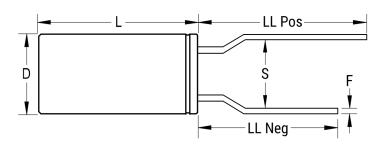
SeriesESEDielectricAluminum ElectrolyticDescriptionSingle Ended, Aluminum ElectrolyticRoHSYesLeadFormed To 5mmAEC-Q200No
