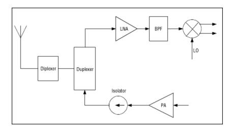
The front-end gain must be high enough to overcome the noise contribution of the following circuits, which may otherwise degrade the receiver's sensitivity. This gain is constrained by the strong out of band unwanted signals and the linearity of the following circuits. If the front-end gain is too high, the mixer will overload and compromise the performance. An LNA with a 14dB to 16dB gain step is a proper selection for both bands.
