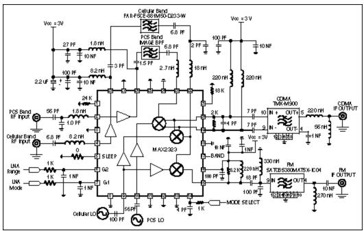
Figure 2. Application circuit of the MAX2323.
