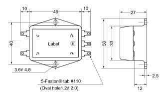
Specifications Voltage AC 250 VAC 1500 VAC Withstanding Voltage 1 Min. Line to Voltage Ground Rated Current 3 A (AC/DC) Temperature -20/+60°C Range 300 MOhms MIN Insulation 500 VDC 1 Min. Line Resistance To Ground
