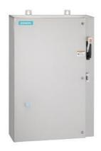
Non-reversing motor starter Size 0 Three phase full voltage Solid-state overload relay OLRelay amp range 0.25-1A 24Vdc coil Combination type 30Amp non-fusible disconnect Encl NEMA type 4X 316 S-steel Water/dust tight non-corrosive Extra-wide enclosure
